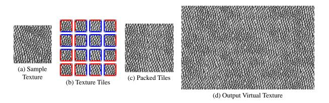
Figure 1: Overview of our system. Given a sample texture (a), we first construct a set of texture tiles [Cohen et al. 2003] (b) so that adjacent tiles have continuous pattern across shared edges. We pack the tiles into a single texture map (c) and store it on a graphics processor. This texture map can then be sampled and filtered via a fragment program to support an arbitrarily large virtual texture (d) without physical storage.
